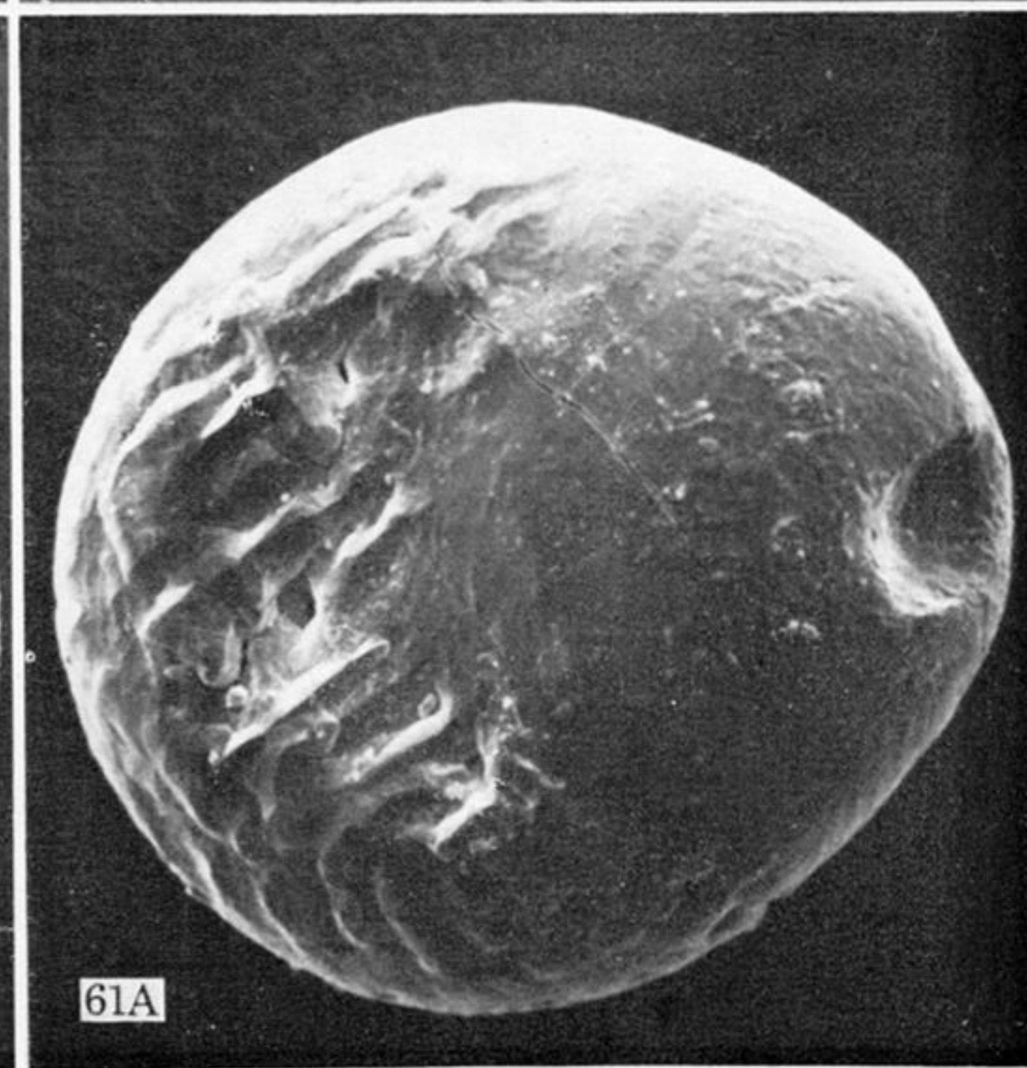
PLATE 11. Iron spherules, ballooned forms and other globular forms.
