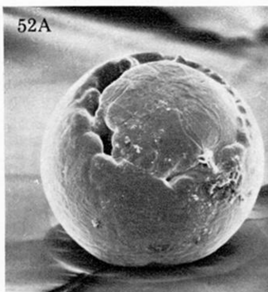
PLATE 10. Iron spherules, metallic globular form: surface details.
