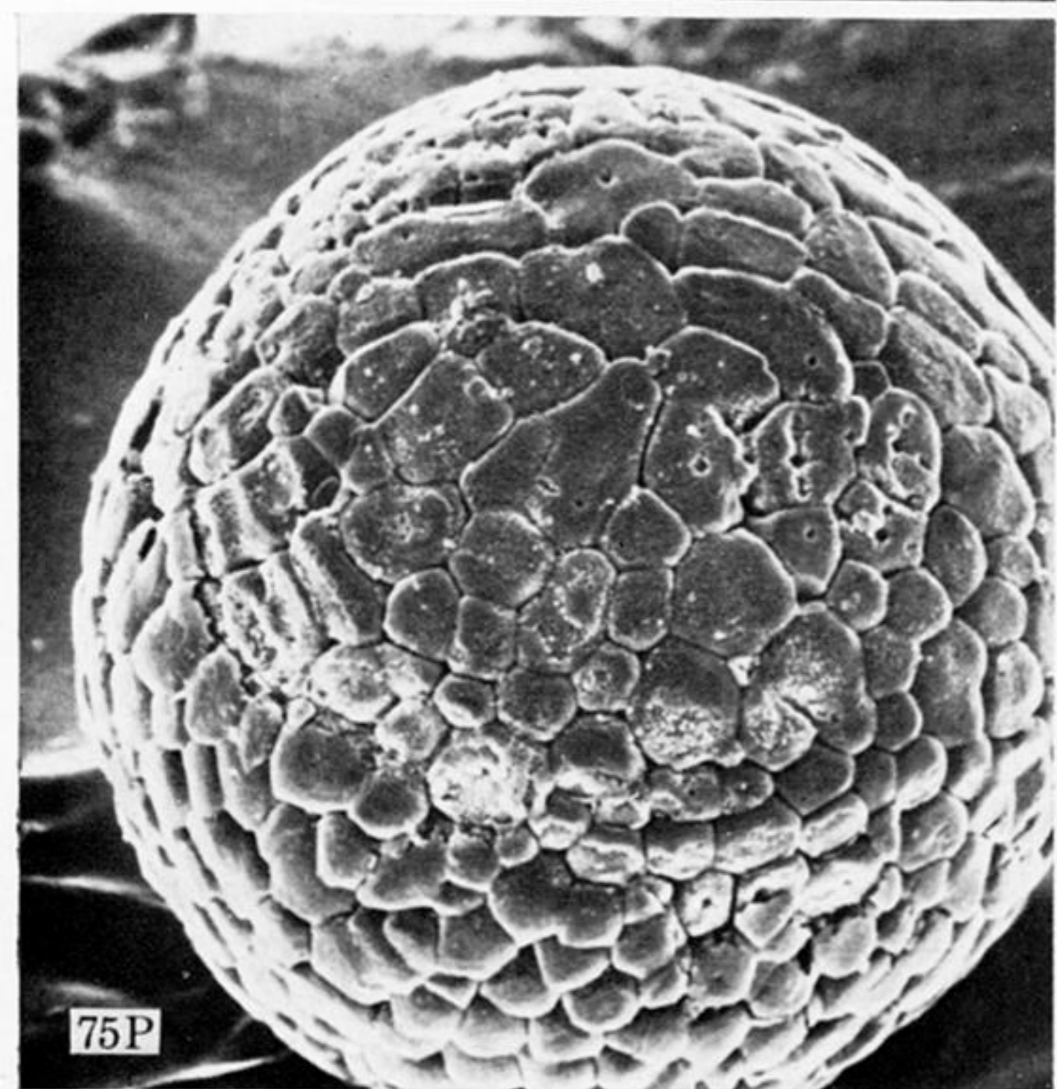
PLATE 14. Iron spherules, the magnetite-wüstite and pure magnetite forms showing large crystals.
